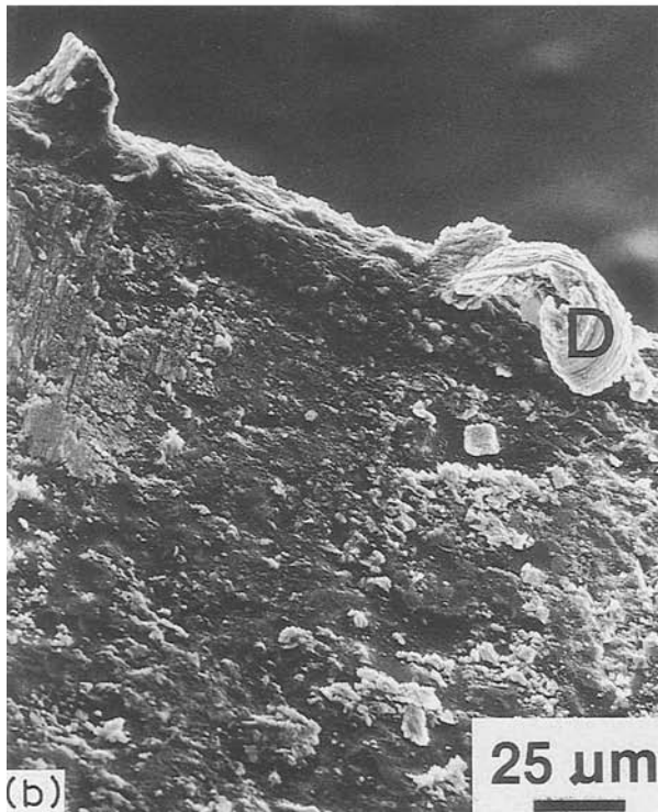
Figure 9 The PCA bracket coated with PEO1 shows the normal PCA surface texture that is partially masked by a porous, low molecular weight polymer (a). The slot edge demonstrates \beta -Ti arch wire debris (D in (b)).
